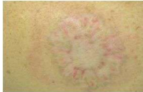
Frequency Double Q-Switched Nd:YAG Module after 8 Tx. 700 mJ/pulse @ 10 Hz.
